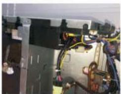
Outdoor main board reverse installation design, better anti-fungus, better duct and wind prevention, especially suitable for GCC countries.
